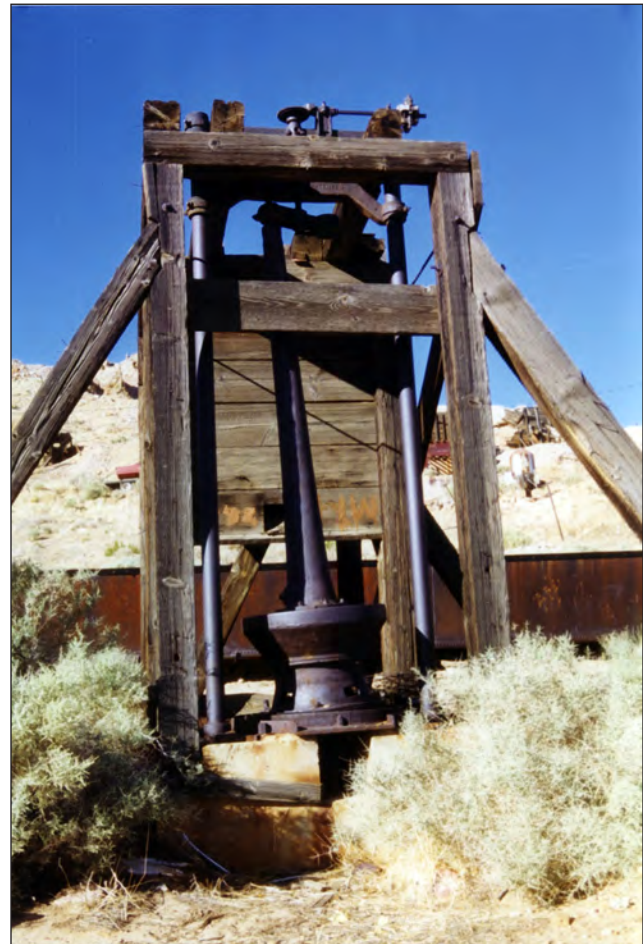
Figure 39. Gibson crusher, used at the Elephant Eagle mine (now part of the open pit) in the 1930s. Richard Graeme, geologist with Golden Queen Mining Company, worked to donate this rare Gibson Gyratory Crusher to the Mojave Desert Heritage and Cultural Association (MDHCA) at Goffs, California in 1999. It was restored and now operates. Photo by Bill Fullerton, MDHCA
