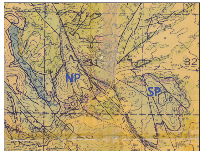
Figure 14. Christensen's Map of the area around the Painted Gorge Fault and the two plugs. "NP" - northern plug. "SP" - southern plug. Note the breccia along the north-northwest Painted Gorge fault that crosses the Painted Gorge drainage and continue on the west side of the southern plug. Christensen considers the breccia in the plus to be fault related. Note also the other north-northeast faults that cross the Painted Gorge drainage and continue south of the southern plug.
