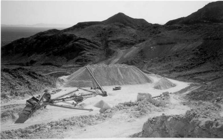
Figure 6. Amboy limestone quarry. Upper photo: haul truck being loaded with pharmaceutical grade limestone ore, 1240 bench, blast hole drill working on bench above. Lower photo: crusher and crushed ore stockpile.
