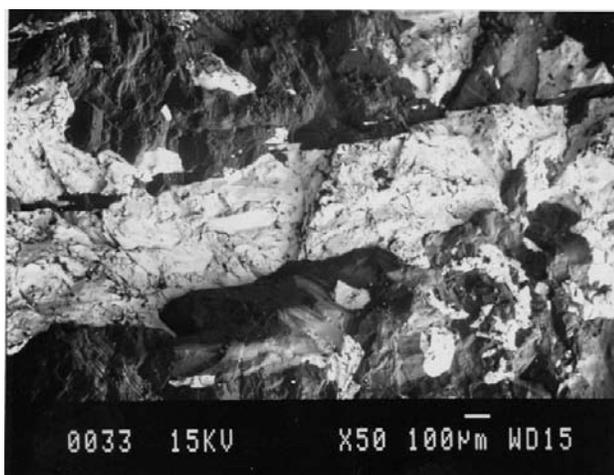
**Figure 2.** Thin vein containing a mixture of friedrichite and gustavite in calcite from the St. Charles mine. BSE image.
