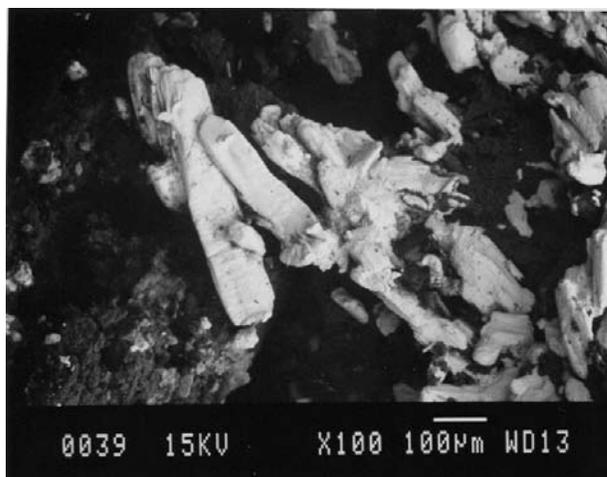
**Figure 9.** Typical combination of junosite and krupkaite grains exposed by etching from limestone. SEM image.
