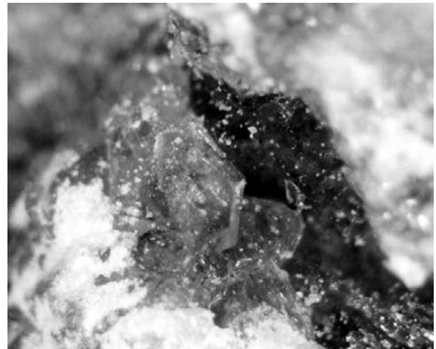
Figure 4. Typical blocky purple coquimbite crystals, to 6.8 mm, associated with brown römerite in fine-grained coquimbite.
