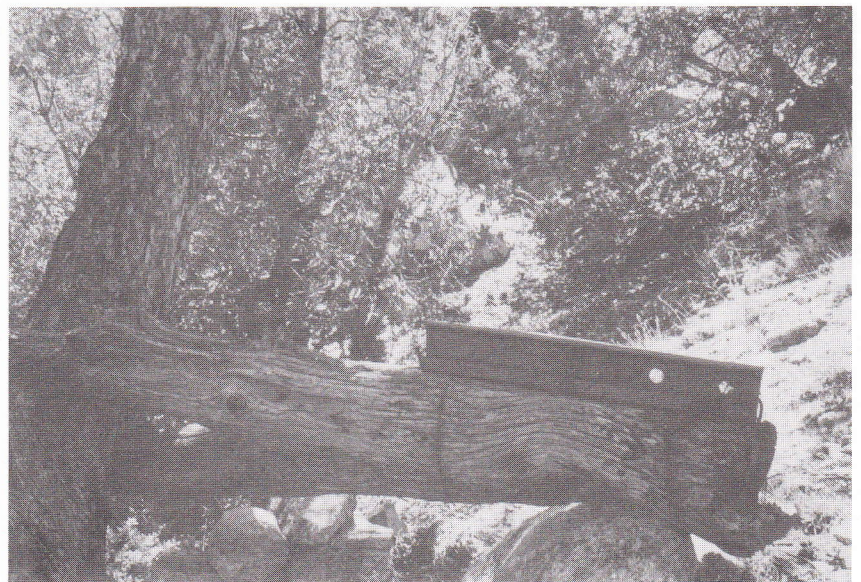
Figure 2. Anvil made of railroad track, wired to forked log and braced by tree and rock, at the New York Peak Prospect. R.E. Reynolds photograph.
