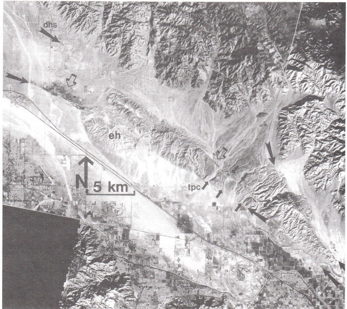
Figure 3. Landsat Thematic Mapper mosaic of the Indio Hills region, California. Large black arrows mark the three major right-slip faults that cut the uplift: from southwest to northeast, Banning, Mission Creek, and Indio faults. Small black arrows depict right-slip offset of canyons along the strike-slip faults, and open arrows point to where the strike-slip faults act as barriers to groundwater flow. eh , Edom Hill; dhs , Desert Hot Springs; tpc , Thousand Palms Canyon. Images were processed at Chevron Oil Field Research Company, La Habra, California.
